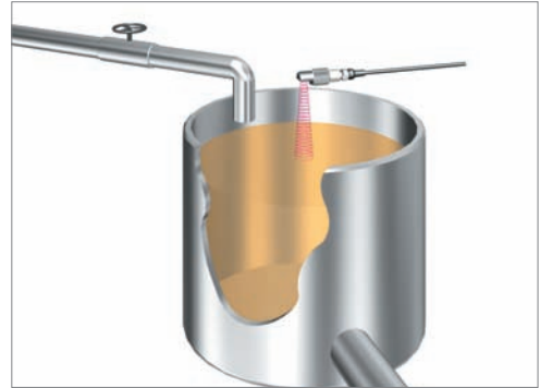
●Inspection of Solvent Tank Levels
