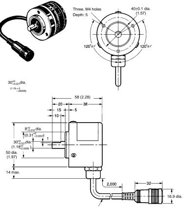
Oil-proof PVC, shielded 12-conductor cable (7/0.18 dia.)
