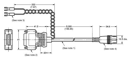
Note: 1. 6-dia. oil-proof PVC, shielded 12-conductor cable (7/0.18 dia.); standard length: 5 m
